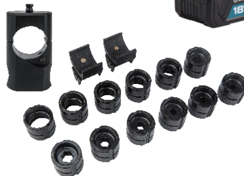
Interchangeable Crimping Dies: 16,25,35,50,70,95,120,150,185,240,300,400mm 2
